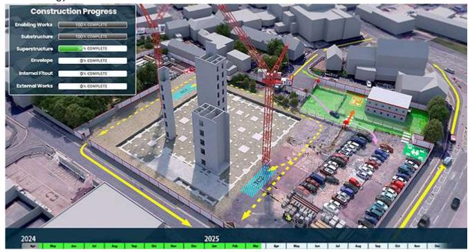
A 4D construction sequence or 4D phasing animation allows construction programmes, schedules, and logistics strategies to be represented graphically. They are simulated by producing 3D models of the scheme and adding a 4th Dimension – Time. These build sequences provide the opportunity to visualise the proposed construction methodology and display knowledge and understanding of the project, demonstrating to an audience the technical details in a clear and precise way.
